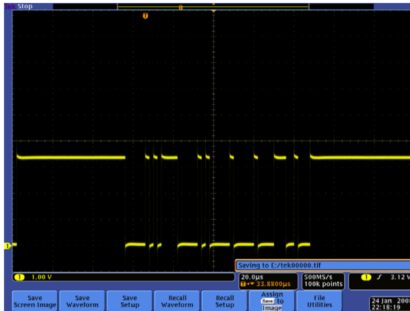
Figure 3. Data Frame Periodically Sent by the HS-CAN Node – Yellow Trace = TxD Signal Coming from the CAN Controller
